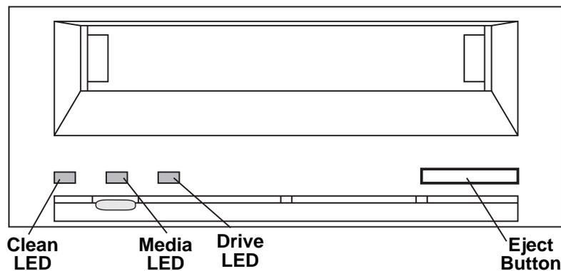
Figure 19. Front panel of internal Scorpion 40 (external drive is similar)
