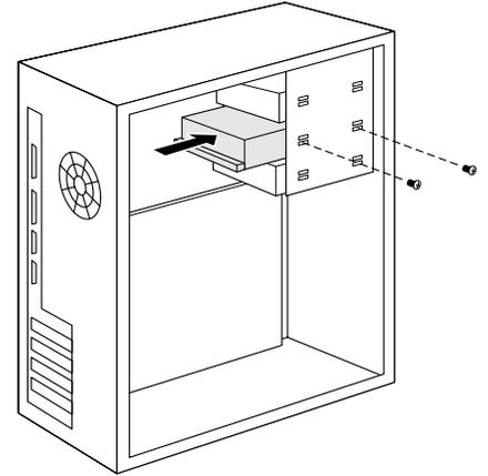
Figure 8. Mounting a drive
