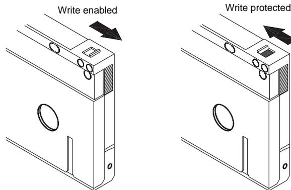
Figure 18. Write-protect tab on a DDS cartridge
