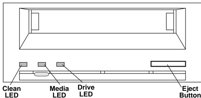
Figure 19. Front panel of internal Scorpion 40 (external drive is similar)
