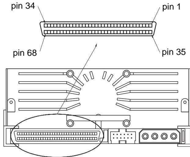
Figure 11. Interface and power connectors on internal Scorpion 40
